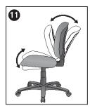
Dual FunctionTwo levers modify:Angle of back relative to seat
